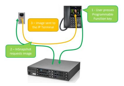
The setup of each Programmable Function key and the target image source is also done via a simple user interface accessed via a Web browser, this would usually be done by the installer or system administrator.
